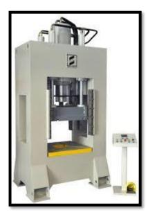
The round blank is next put into this machine and the machine will punch out the desired shape of the frying pan.
