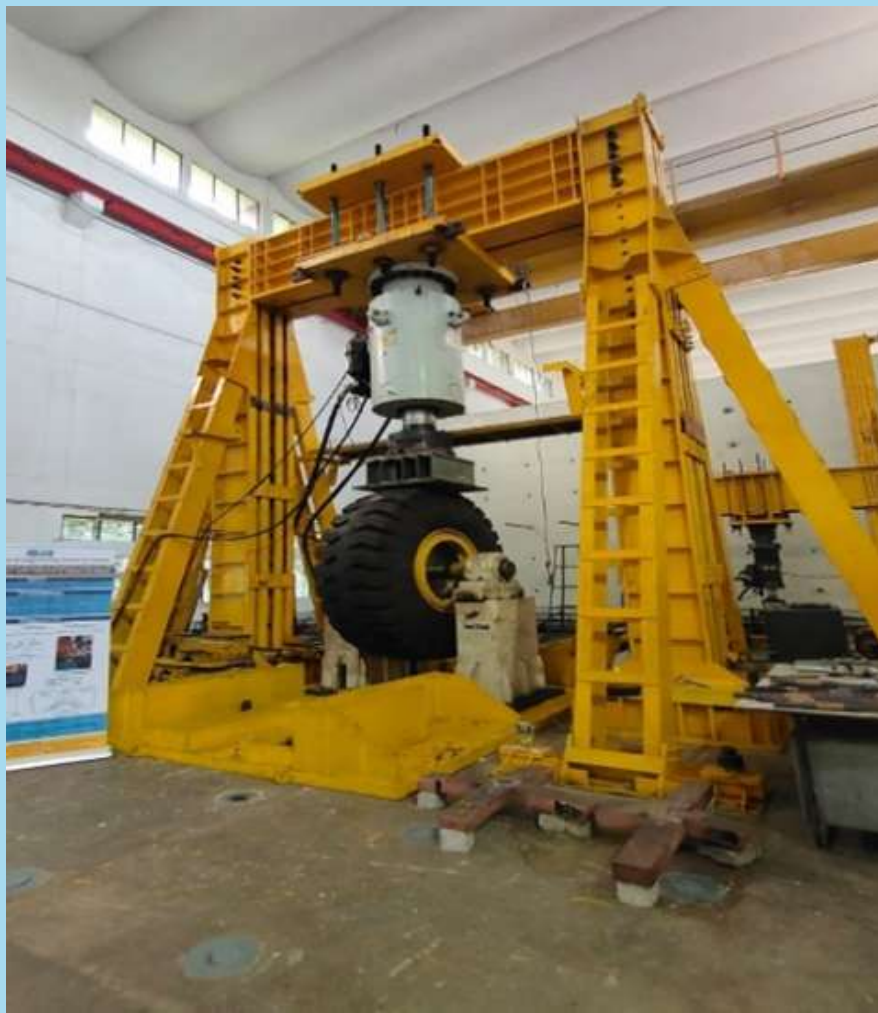
Earth moving tyre under static loading (Fatigue and Fracture Lab)
