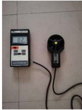
Measurement of wind velocity in m/s using Anemometer
