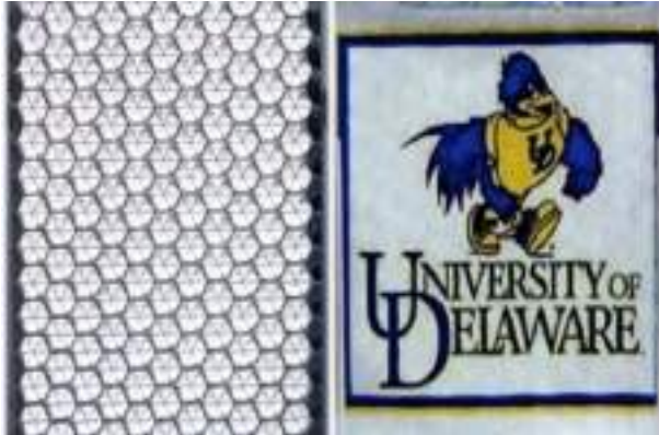
The glass in its retroreflective state (left), and its clear state (right) (Credit: Keith Goossen, University of Delaware )
