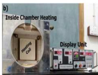
Pin-on-Disc Setup (a) Chamber heating (b) Heating Coil and Display unit
