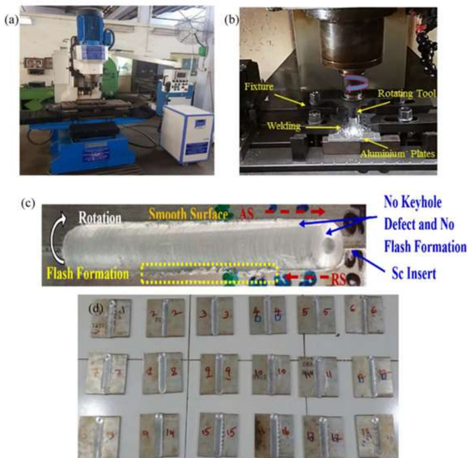
Figure 2. (a) Friction stir welding machine (b) FSW Process (c) Welded area of the plate (d) 17 trails and confirmation welded samples.
