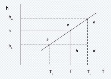
In the above diagram the points a and e represent points that are in the table and point c is the position at which the properties are required. If the variation is linear, that is, if ae is assumed to be a straight line, then using the principle of similar triangles:
