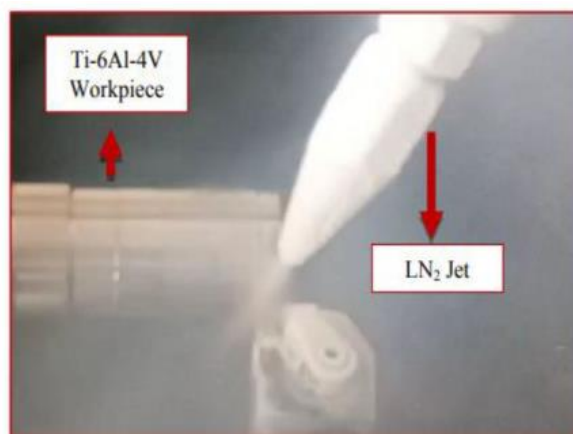
Figure 4. Photographic view of LN 2 jet on the tool-workpiece interface (Khan et al., 2019).
