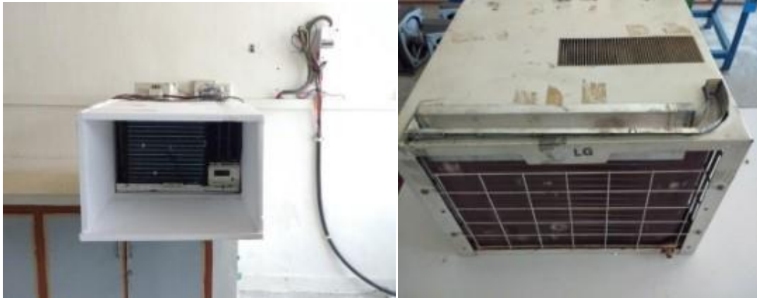
Figure 15: (LEFT) Evaporator side of the unit, (RIGHT) Condenser side of the unit with condensate water spray arrangement
