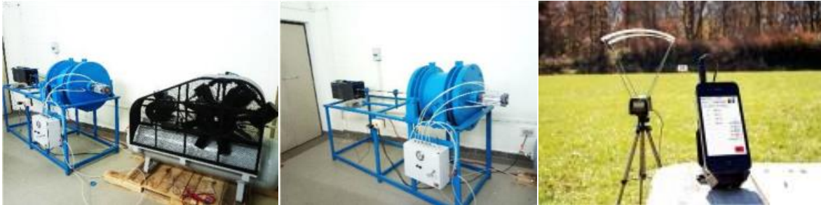
Figure 31: (LEFT) Gas Gun Setup with compressor (MIDDLE) Gas Gun Setup (RIGHT) Ballistic Chronograph
