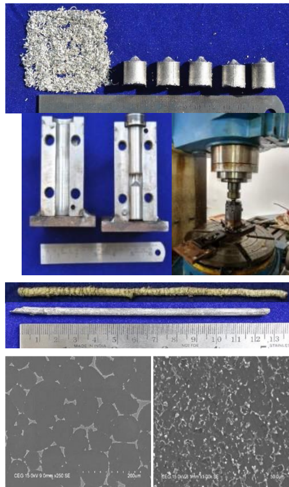
Figure 9: Recycling of Magnesium Chips using Friction Extrusion
