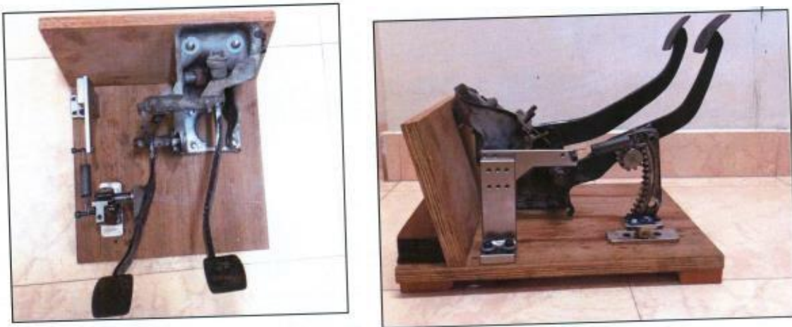
Figure 5: Slow release clutch mechanism
