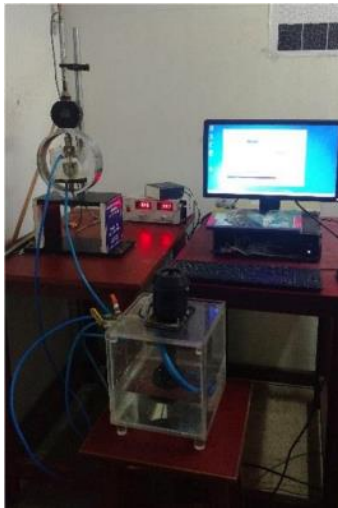
Figure 28: Stress Corrosion Cracking Setup
