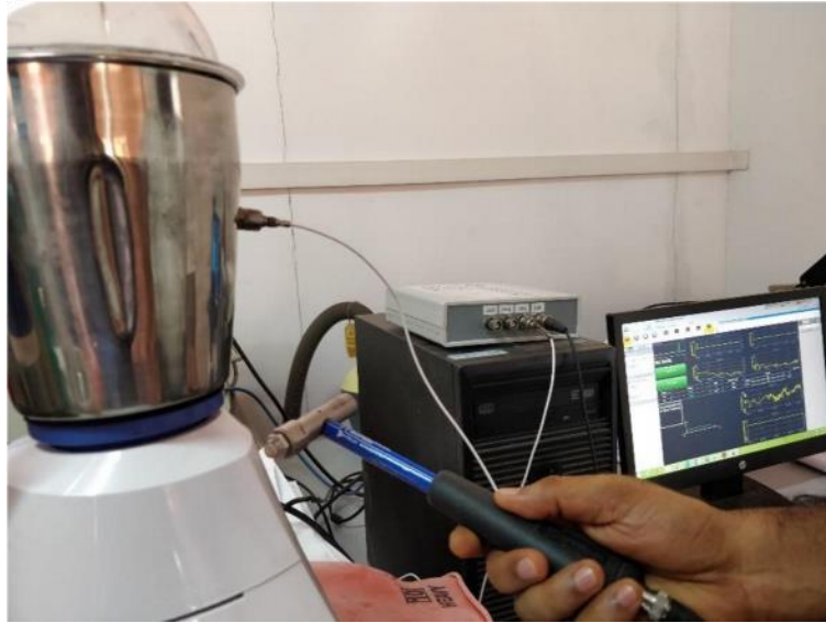
Figure 30: Mixer being tested for vibrations
