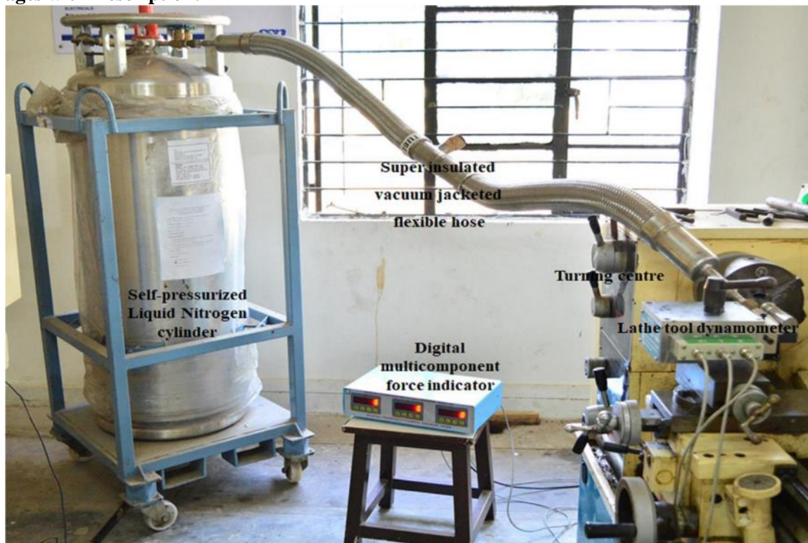
Figure 22: Cryogenic cooling unit for hard to cut materials.
