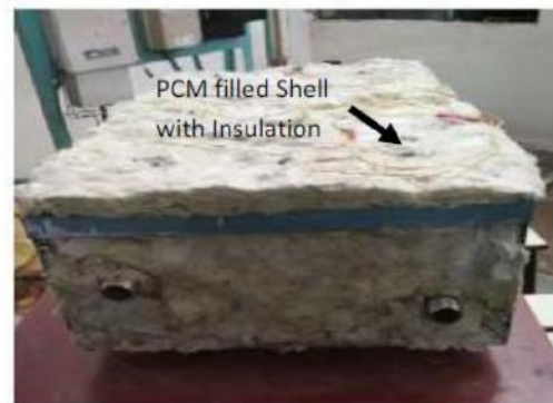
Insulated assembled unit after filling with PCM
