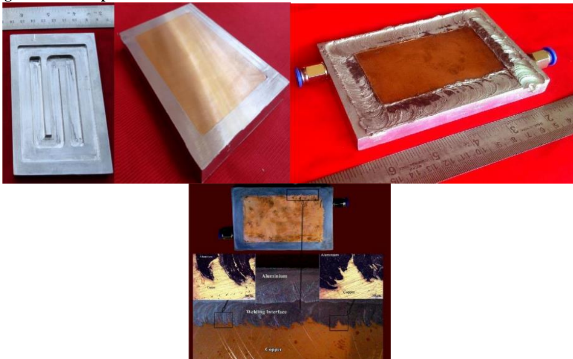
Figure 8: Cold Plate or Heat Sink
