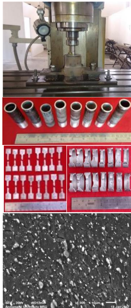
Figure 10: Friction stir back extrusion of ZE41 magnesium alloy
