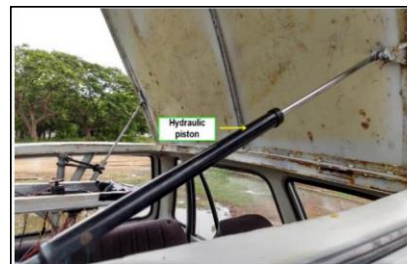
(b) roof opening Mechanism
