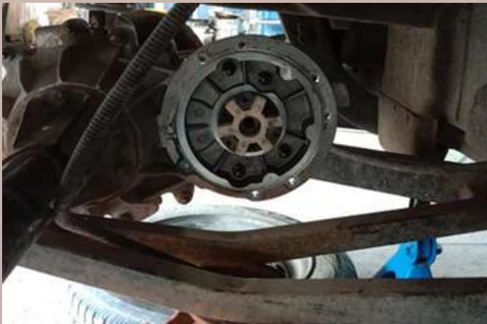
Drive housing with differential gear set up and positioned drive
