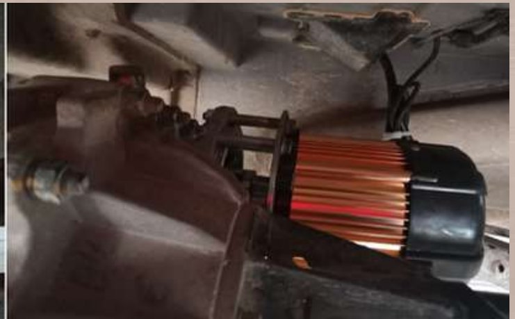
Drive housing with differential gear set up and positioned drive
