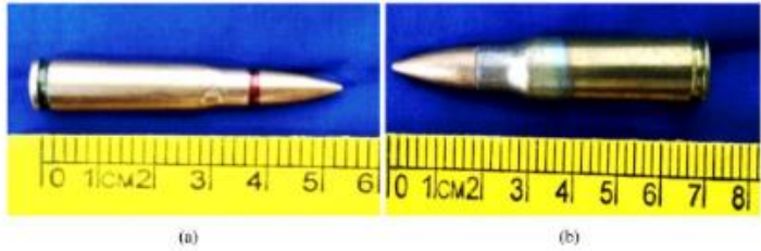
Fig. 3. Photograph of projectiles (a) 7.62 mm x 39 mm steel core projectile; (b) 7.62 mm x 51 mm lead core projectile.
