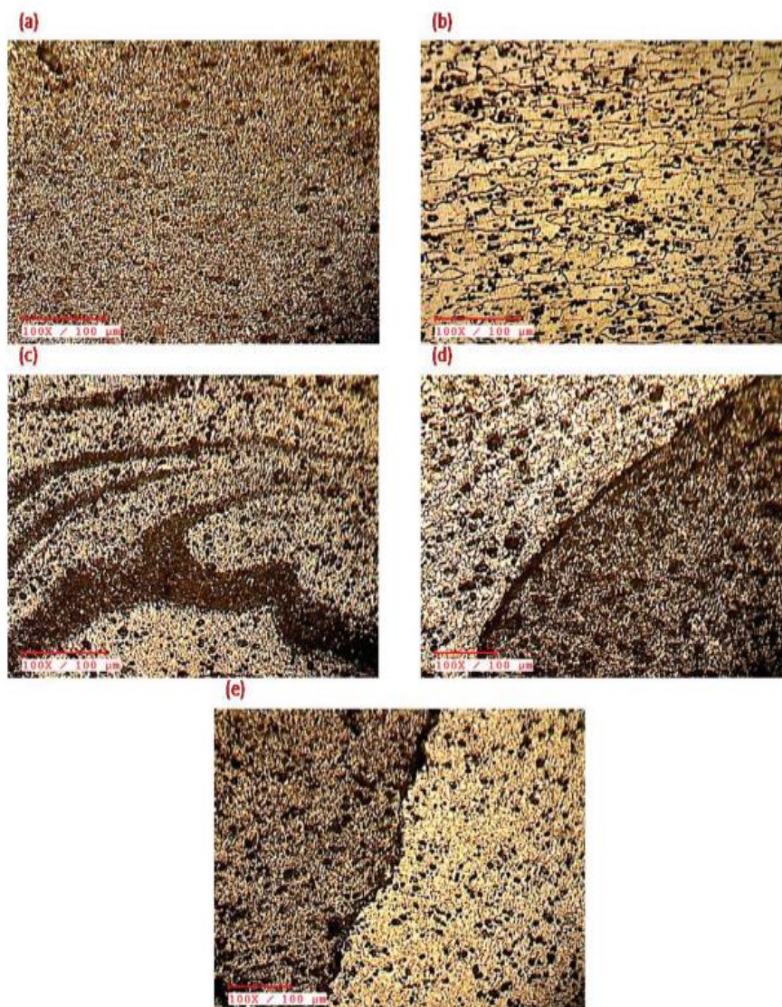
Figure 4. Optical microscopy (a) 5083 base metal; (b) 6061 base metal; (c) weld nugget – square pin; (d) weld nugget – threaded cylinder; (e) weld nugget – tapered cylinder.
