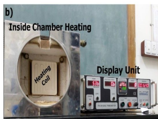
Pin-on-Disc Setup (a) Chamber heating (b) Heating Coil and Display unit
