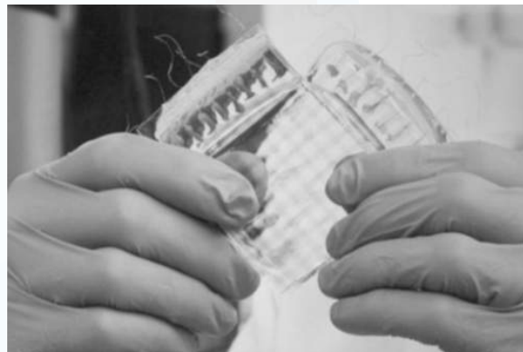
Figure 4. Sensor for measuring mechanical deformation can be stretched in all directions and then take its original shape
