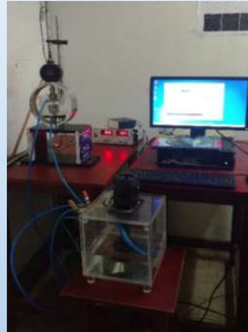
Stress Corrosion testing
