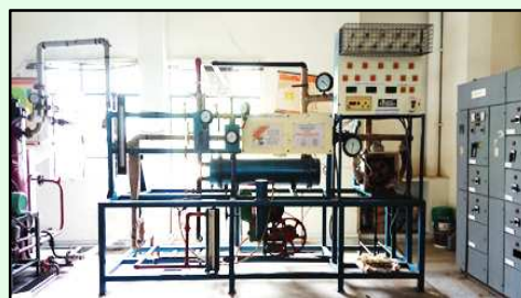
Steam Boiler-turbine unit
