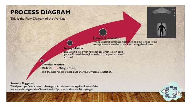
The shell of the suit is proposed to be made of recycled plastic bottles for making it eco-friendly. A gyroscopic sensor is used that detects the acceleration during the fall time and triggers the spark for the chemical reaction which inflates the Airbag by filling the Nitrogen gas.
