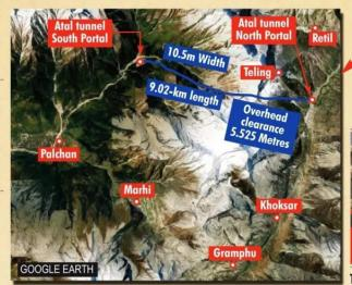
Shaped like a horse-shoe, the tunnel is double-laned and in a single tube. It has a roadway of 8 metres. Speed inside the tunnel to be 80 kmph A fire-proof emergency exit tunnel has also been built within the main tunnel itself. This emergency tunnel is 3.6 metres by 2.25 metres.
