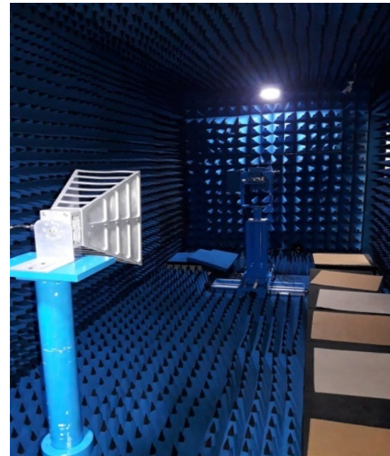
Anechoic Chamber (7 m x 3 m x 3 m)
