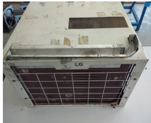
Condenser side of the unit with condensate water spray arrangement
