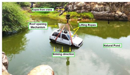
(c) Full scale testing of car –orientation1
