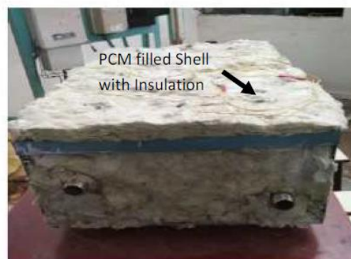
Insulated assembled unit after filling with PCM
