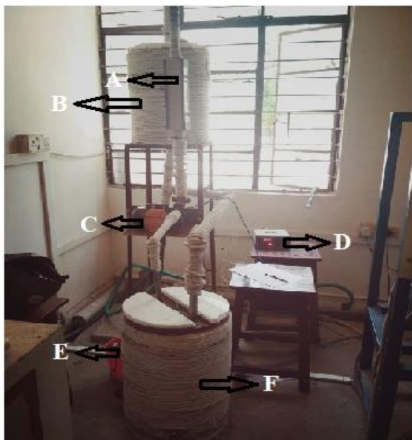
Photographic view of TES tank integrated with Temperature bath
