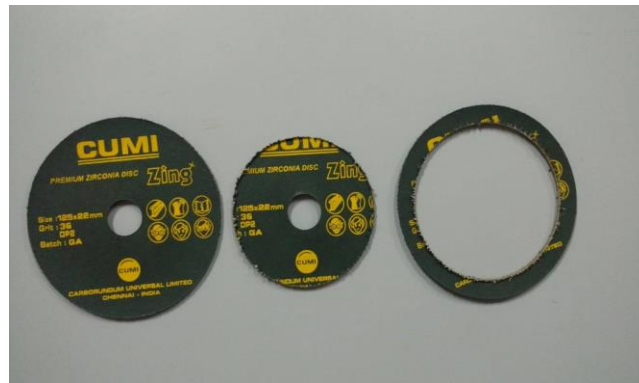
Figure showing original disc, recovered disc and trimmed edge
