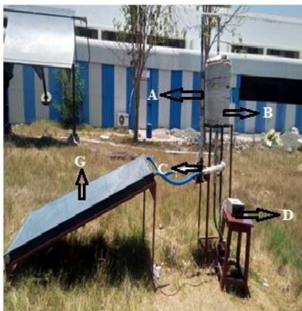
Photographic view of TES tank integrated with solar flat plate collector
