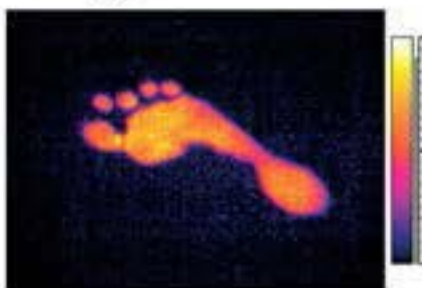
IR image showing the temperature distributions of bare foot walk
