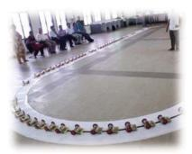
running 100 line-tracing robots simultaneously on a single arena. Line tracing is a phrase familiar among all the robotics enthusiasts where in, an autonomous vehicle, called a bot follows a black line of a pre decided thickness.
