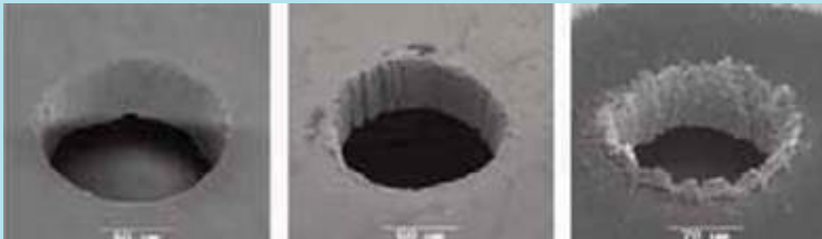
Fig. 2: Micro drilling - Aluminium Ti: sapphire, 120fs a) air b) vacuum c) Nd:YAG, 100ns
