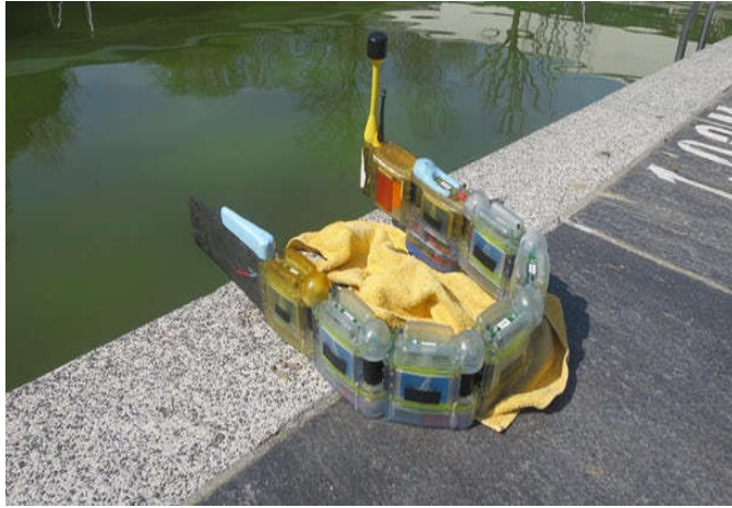
The Snakebot with different modules containing different sensors
