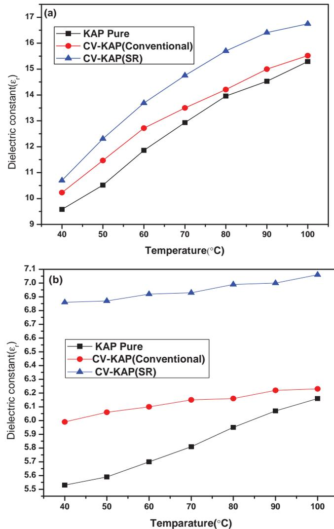
Fig. 6. Temperature versus dielectric constant at (a) 1 kHz (b) 1 MHz.
