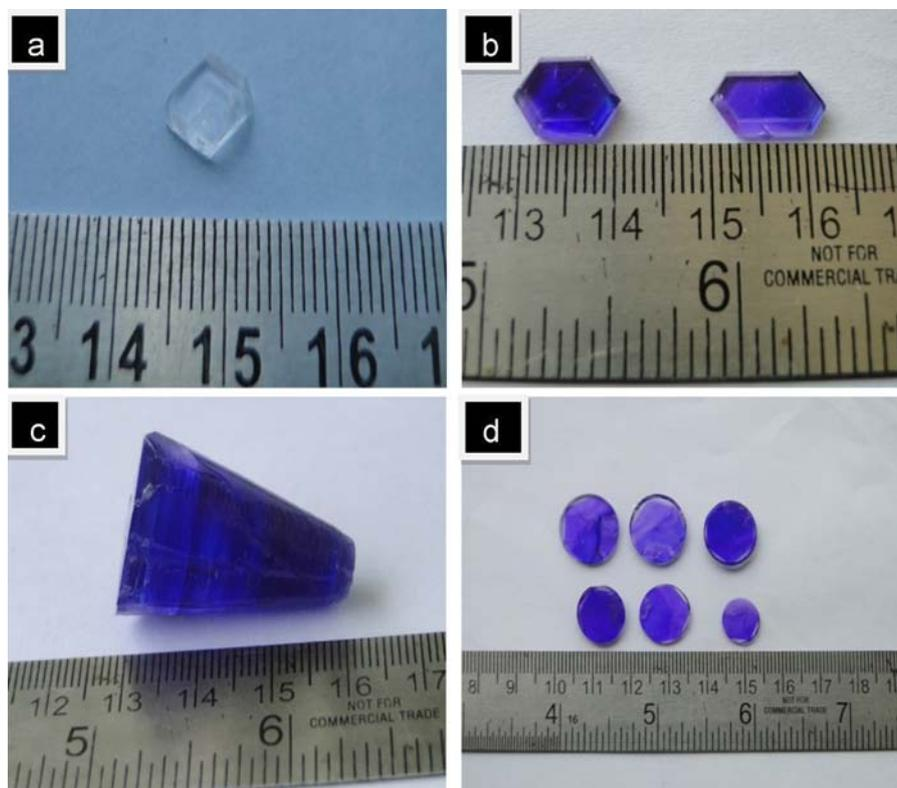
Fig. 1. Crystals grown by (a) conventional method grown pure KAP (b) dye doped KAP (c) SR method grown dye doped KAP (d) cut and polished crystal ingot.
