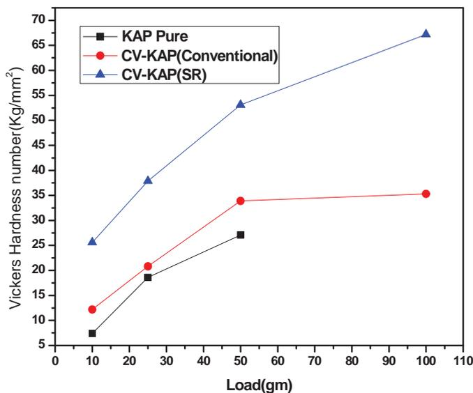
Fig. 4. Vicker's hardness measurement for dye KAP crystals.
