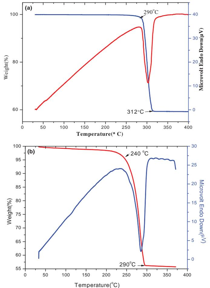
Fig. 5. TG-DTA curve of (a) KAP pure (b) dye doped KAP crystal.
