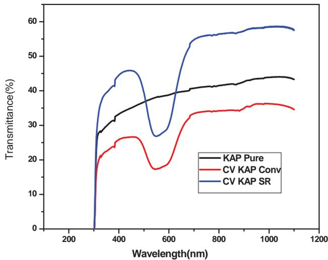
Fig. 2. UV-vis analysis of pure and dye doped KAP single crystals.
